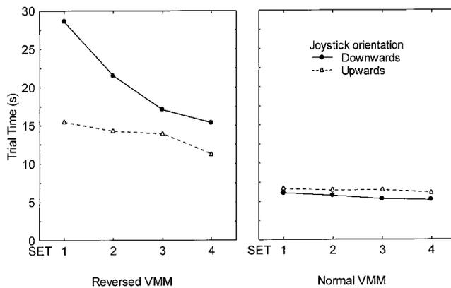
**Figure 7.** Trial time for the manipulation task as a function of the visual-motor mapping (VMM), the orientation of the joystick, and the experimental set.
