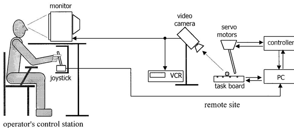
**Figure 3.** A schematic depiction of the experimental apparatus.
