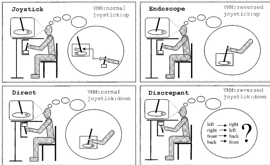
**Figure 2.** The four design alternatives of a hand-controller in endoscopic teleoperation and their corresponding mental models.
