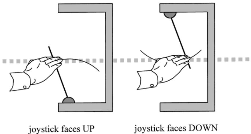
**Figure 4.** A schematic depiction of the construction that holds the joystick. It ensures a similar grip in both the upward and the downward orientations of the joystick.
