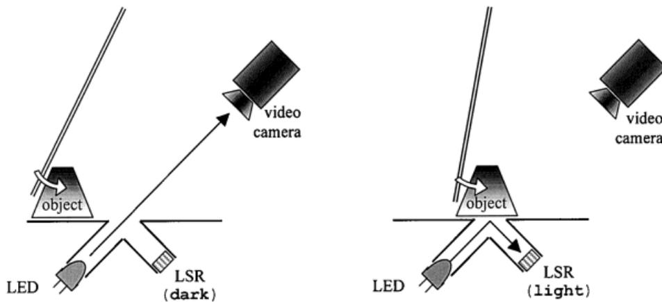
**Figure 6.** The object-detection mechanism that was implemented in the task board.
