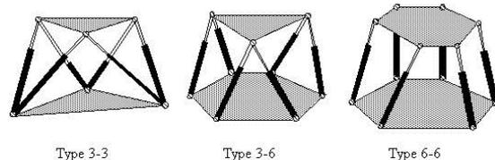
Figure 1: Three types of parallel mechanisms
