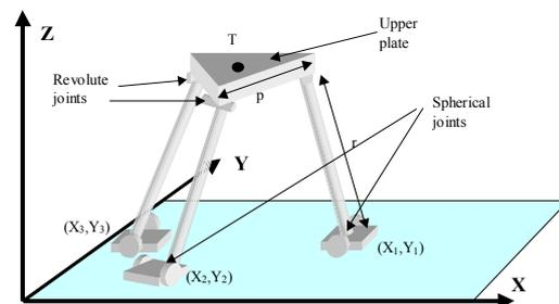
Figure 4: Schematic description of the mobile parallel mechanism
