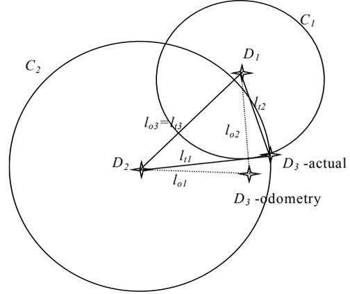
Figure 7: Determining the position of  $D_3$  by the intersection of  $C_2$  and  $C_1$
