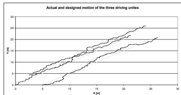
Figure 10: Simulation of random odometric error for three driving units simultaneously
