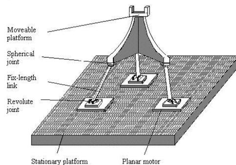
Figure 2: Semi-mobile parallel mechanism [Ben Horin and Shoham, 1996]
